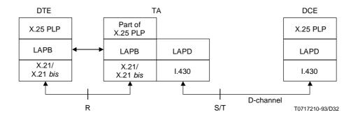
FIGURE IV.1/X.31 Example configuration in the idle phase, non-transparent at layer 3
