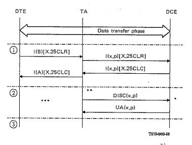
\* The D-channel logical link is disconnected, only if the cleared virtual call was the last one via that link.
