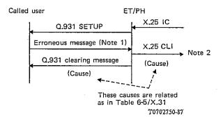
Note 1 — This figure only applies to the case where the erroneous message results in a Q.931 clearing message. See § 6.4.3 for more information. Note 2 — This message would be sent after the expiry of timer T303 on a multipoint interface.
