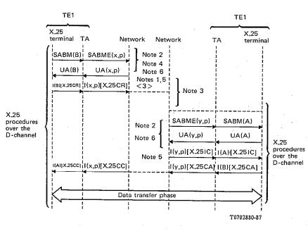
Note 1 – When the called side establishes the call using B-channel access, the message sequence will continue as from point <1> in Figure III-1/X.31.
