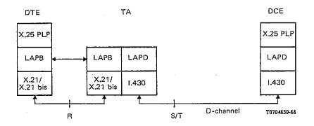
FIGURE IV-2/X.31 Example configuration in the idle phase, transparent at layer 3
