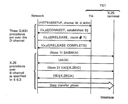
Note 1 – The network establishes the link layer in the B-channel if it is not already established. See § 6.3.
