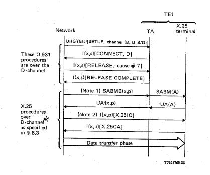
Note 1 – The network establishes the link layer in the D-channel if it is not already established. See § 6.3. The network starts timer T320, if implemented. Note 2 – The network cancels timer T320, if implemented and running.
