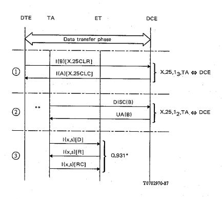
\* The B-channel is cleared, only if the cleared virtual call was the last one via that B-channel.
