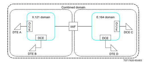
NOTE - This figure is a functional domain diagram and is not intended to imply a real internetwork implementation.
