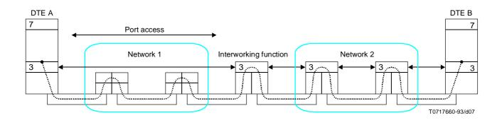
FIGURE 7-2/X.301 QOS Reference Points in an example of interworking by port access
