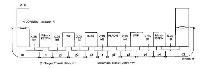
The labels (a), (b), (c), (d), (e), (f) and (g) represent the various points between the entities involved in the scenario shown above at which the transit delay information is visible in the protocol information.
