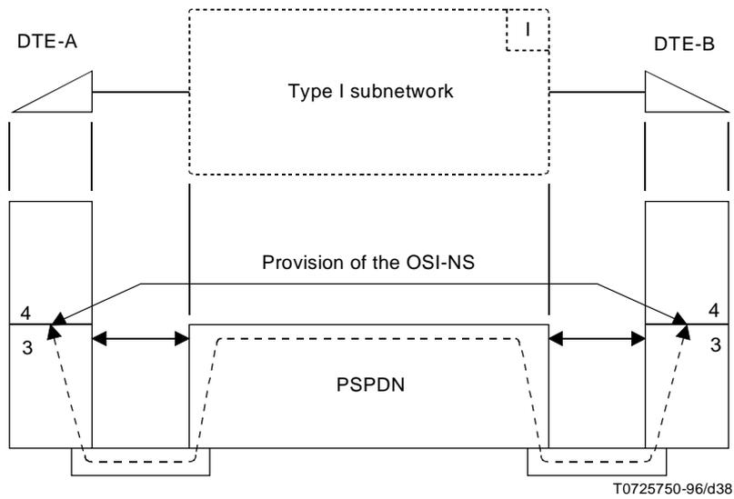
**Example:** PSPDN functionality for connection establishment, data transfer and connection release
