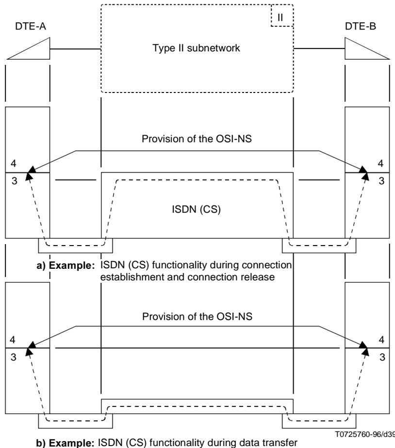
**a) Example:** ISDN (CS) functionality during connection establishment and connection release
