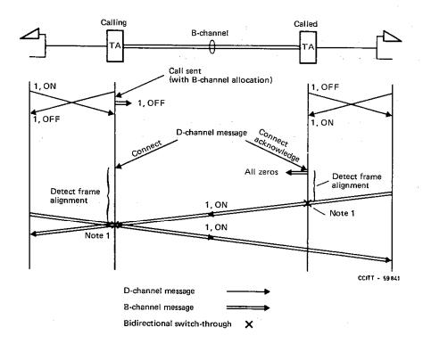
Note 1 — The TA shall perform connect-through after detecting frame alignment and completing delivery to the terminal of any DCE-provided information.
