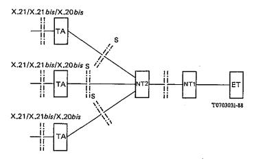
TA Terminal adaptor NT Network termination ET Exchange termination
