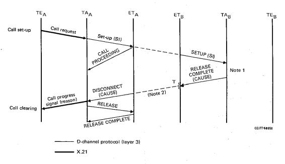
Note I-RELEASE COMPLETE message including the appropriate case code, is sent by a TA supporting a terminal which is compatible with information contained in the SETUP message, to indicate that the call cannot be accepted at this time for the following reasons: controlled not ready, uncontrolled not ready, busy condition of the called terminal, etc.
