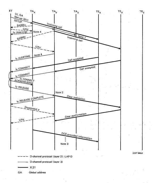
Note 1 — TAz does not respond to the SETUP message because it is supporting a terminal which is not compatible with the calling terminal. However, TAz may alternatively respond with a RELEASE COMPLETE message with the cause "incompatible destination" (#88).
