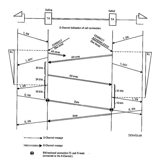
Note — The TA will only indicate ready for data after completing delivery to the DTE of any DCE provided information.
