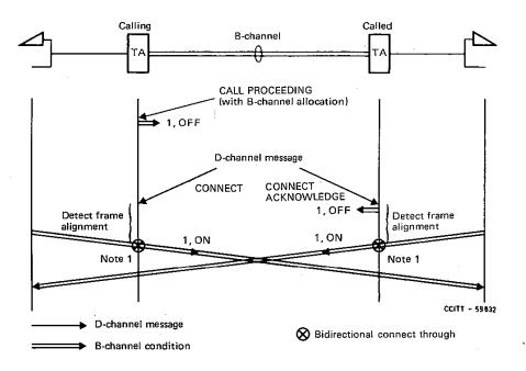
Note 1 — The TA will perform connect-through after detecting frame alignment and completing delivery to the terminal of any DCE-provided information. To guarantee the correct ready for data alignment, through-connection must be performed immediately before the C lead is scanned.
