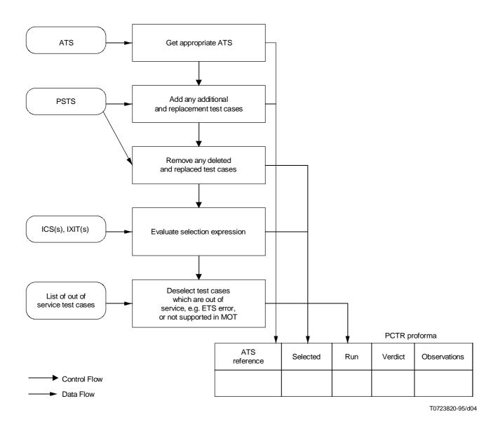
$\label{eq:FIGURE} FIGURE~4/X.294$  Test selection process and listing test cases in the PCTR proforma
