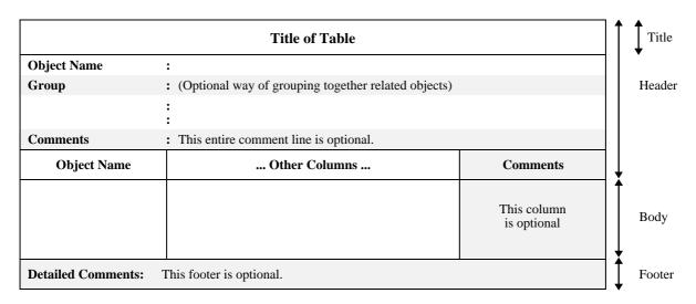
Figure 1/X.292 – Generalized layout of a single declaration table
