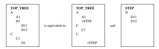
This operation can be performed not only on the main behaviour tree of the Test Case (the root tree) but also on the Test Steps detached from it. The attached tree will either be a local tree or a member of the Test Step Library.
