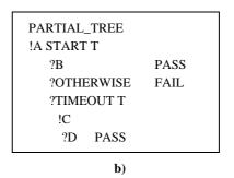
In a) if D is received in response to !A, the test case will assign an erroneous PASS verdict by virtue of the TIMEOUT. This can be avoided by using the OTHERWISE statement.
