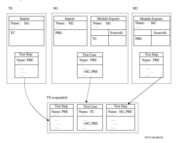
The test step PRE (which is defined in the module M2) is implicitly imported from M1 in TS.
