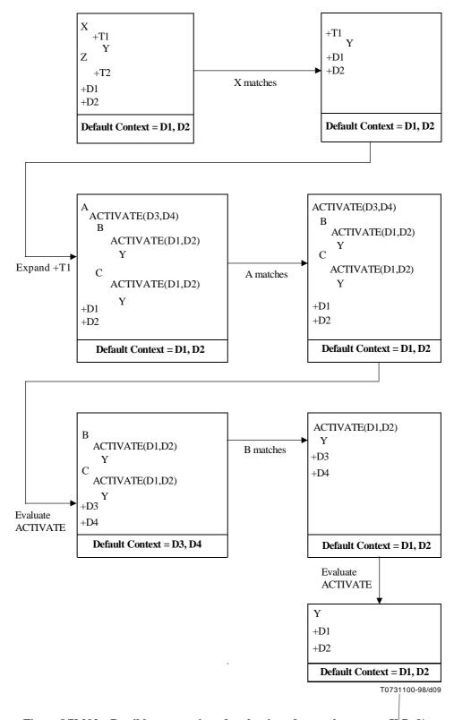
Figure 8/X.292 – Possible progression of evaluation of example test case X<sup>L</sup>Def1
