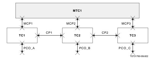
Figure 3/X.292 – Example Test Component Configuration CONFIG1
