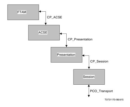
Figure I.6/X.292 – Possible Configuration for Multi-Protocol Testing – Session embedded under FTAM
