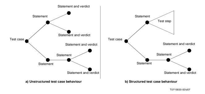
Figure 7/X.292 - Test Case Behaviour Structure
