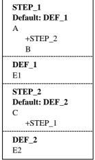
1: STEP\_1 and STEP\_2 attach each other. STEP\_1 has Default DEF\_1. STEP\_2 has Default DEF\_2
