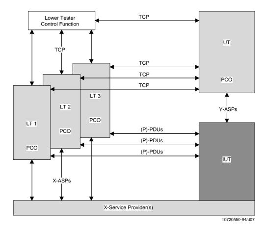
FIGURE 7/X.291 Multi-Party Testing with a single UT
