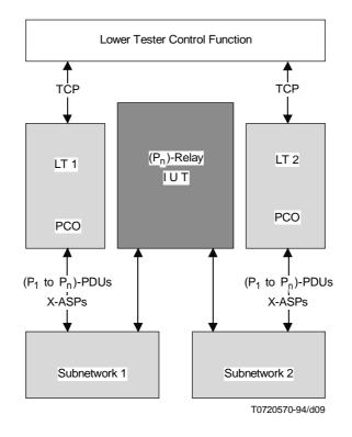
FIGURE 9/X.291 Possible realization with no UT
