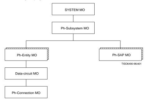
Figure 1 – Physical Layer Containment Hierarchy
