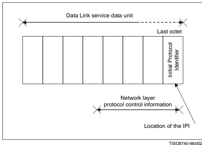
**Figure 2 – Location of the IPI for trailer-oriented protocols**
