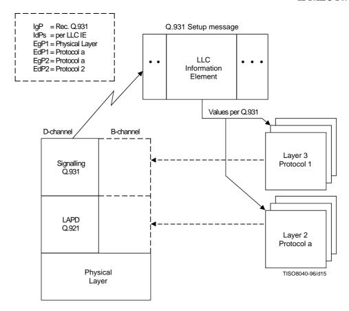
Figure B.2 - Q.931 Identification by Low Layer Compatibility (LLC) Information Element in ISDN
