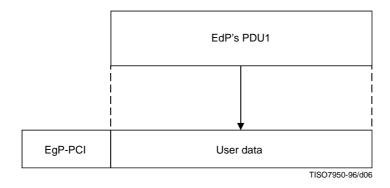
Figure 6 - One PDU of only supported EdP encapsulated in EgP
