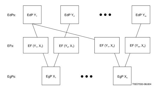
EdP Encapsulated Protocol EF Encapsulation Function EgP Encapsulating Protocol
