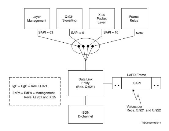
NOTE-Values of Data Link connections on the D-channel that correspond to SAPI values from 32 to 61 are used for Frame Relay service.
