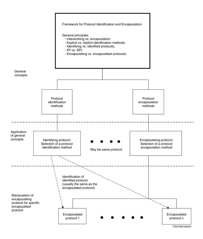
Figure 1 – Framework for protocol identification and encapsulation principles
