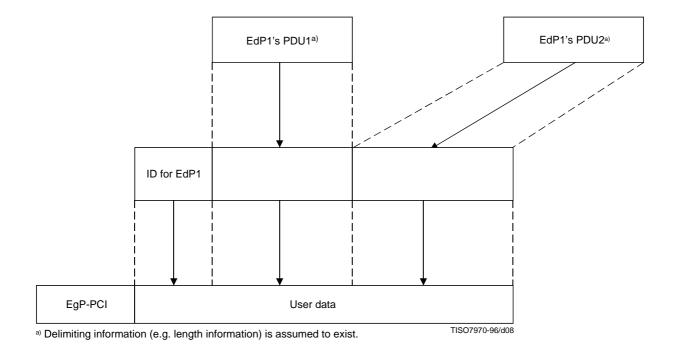
Figure 8 – Multiple PDUs of one of the EdPs encapsuled in EgP
