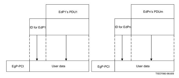
Figure 9-PDUs from multiple EdPs encapsulated in EgP
