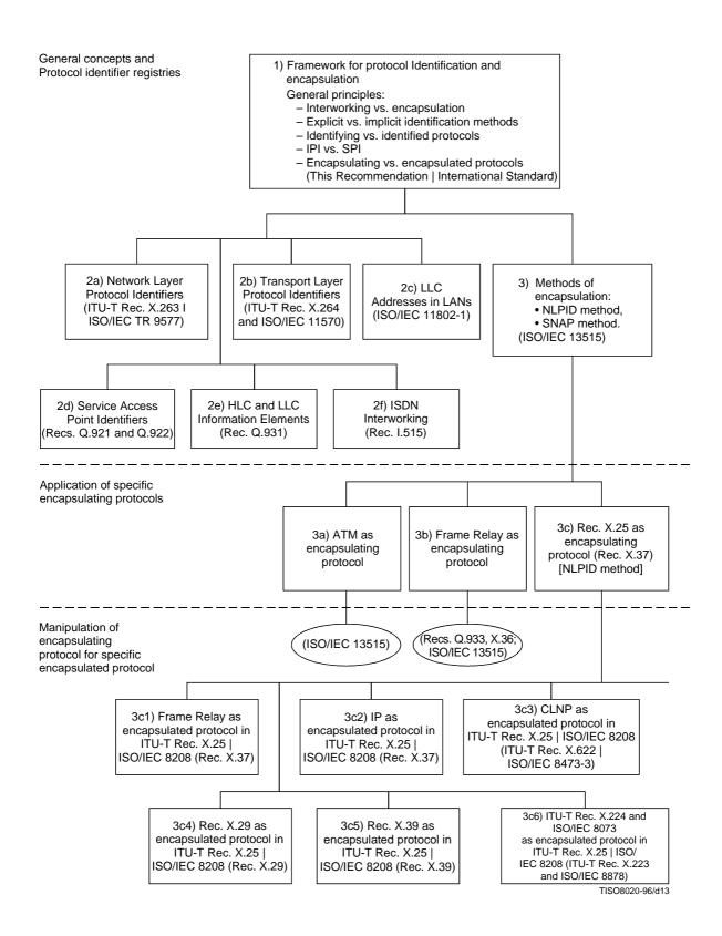
${\bf Figure~A.1-Relationship~of~Recommendations~|~International~Standards~supporting~} \\ {\bf principles~of~protocol~identification~and~encapsulation}$
