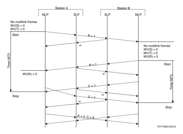
$<sup>^{\</sup>mathrm{a})}$  The SLP frame that acknowledges delivery of the multilink frame with R = 1.
