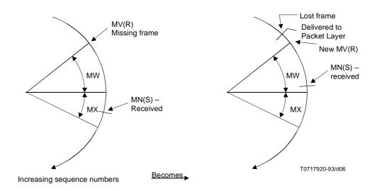
FIGURE 2-4/X.25 **Detecting lost multilink frames**
