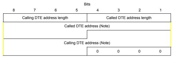
NOTE – The figure is drawn assuming the number of address digits present in the called DTE address field is odd and the number of address digits present in the calling DTE address field is even.
