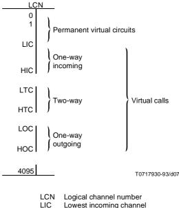
LCN Logical channel number Lowest incoming channel Highest incoming channel Lowest two-way channel Highest two-way channel LoC Lowest outgoing channel Highest outgoing channel
