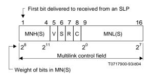
MNH(S) Bits 9-12 of 12-bit multilink send sequence number MN(S) MNL(S) Bits 1-8 of 12-bit multilink send sequence number MN(S)
