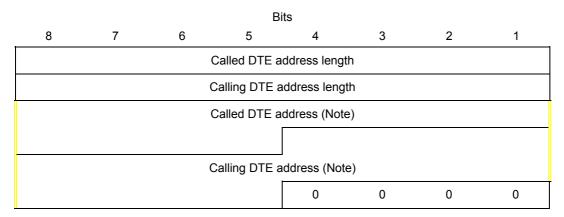
NOTE – The figure is drawn assuming the number of semi-octets present in the called DTE address field is odd and the number of semi-octets present in the calling DTE address field is even.
