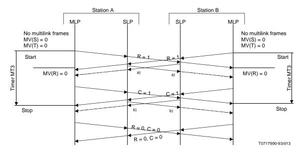
a) The SLP frame that acknowledges delivery of the multilink frame with R = 1.
