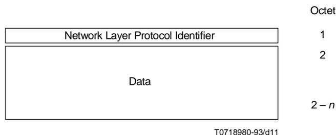
**Figure 10 – Inactive Network Layer Protocol PDU**
