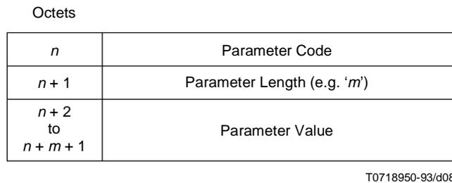
**Figure 7 – Encoding of option parameters**
