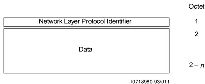
**Figure 10 – Inactive Network Layer Protocol PDU****7.8.2 Network layer protocol identifier**
