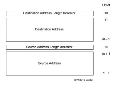
Figure 3 – PDU header – Address part
