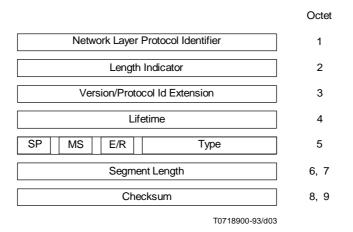
Figure 2 – PDU header – Fixed part
