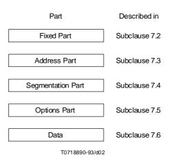
Figure 1 – PDU structure
