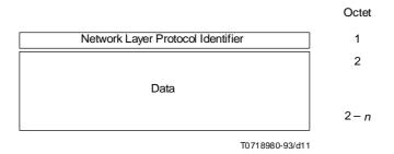
Figure 10 – Inactive Network Layer Protocol PDU
