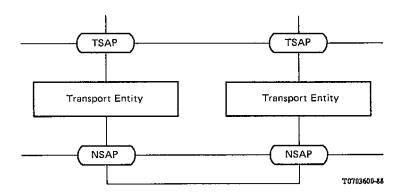
Note — For the purpose of illustration, this figure shows only one TSAP and one NSAP for each transport entity. In certain instances, more than one TSAP and/or more than one NSAP may be associated with a particular transport entity.
