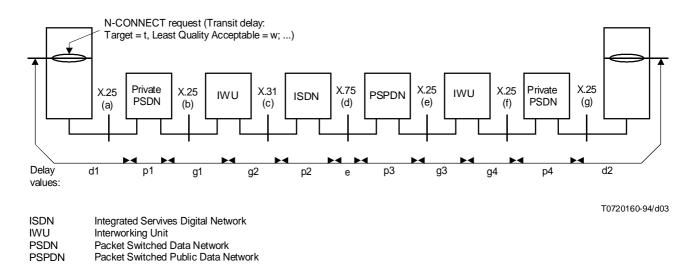
The labels (a), (b), (c), (d), (e), (f), and (g) represent the various points between the entities involved in the scenario shown above at which the transit delay information is visible in the protocol control information.
