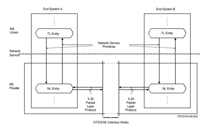
NOTE - This interface consists of zero or more Network Layer entities providing a Network Layer relay function.
