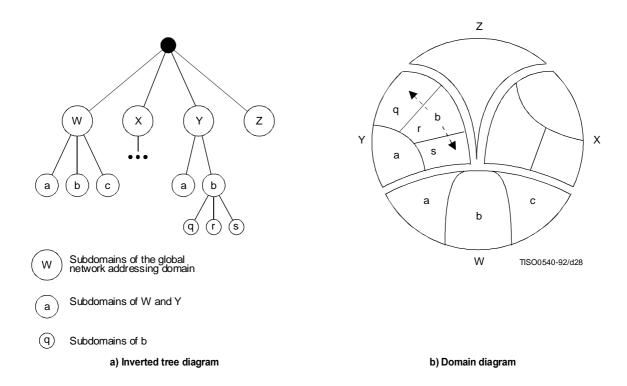
Figure A.4 - Hierarchical structure of NSAP address
