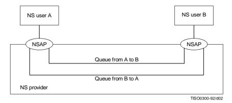
Figure 1 – Queue model of a Network Connection
