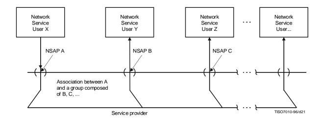
Figure 19b - Model of a multicast network-connectionless-mode transmission
