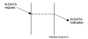
Figure 12 – Sequence of primitives in data transfer
