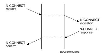
Figure 5 – Sequence of primitives in successful NC establishment
