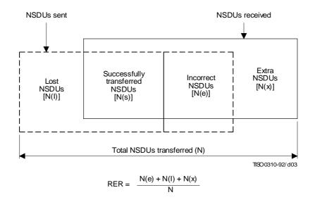
Figure 2 – Components of residual error rate
