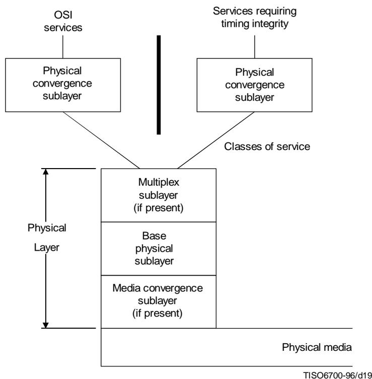
**Figure A.1 – Structure of the Physical Layer**
