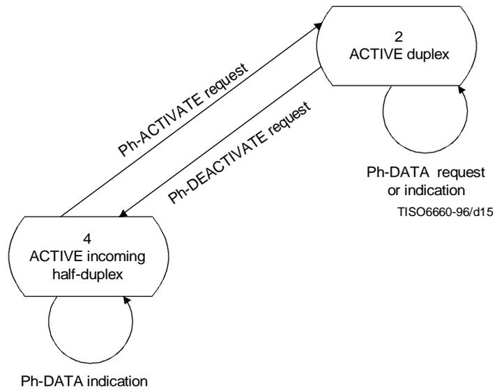
Figure 14 – State transition diagram for half-duplex/duplex mode shift
