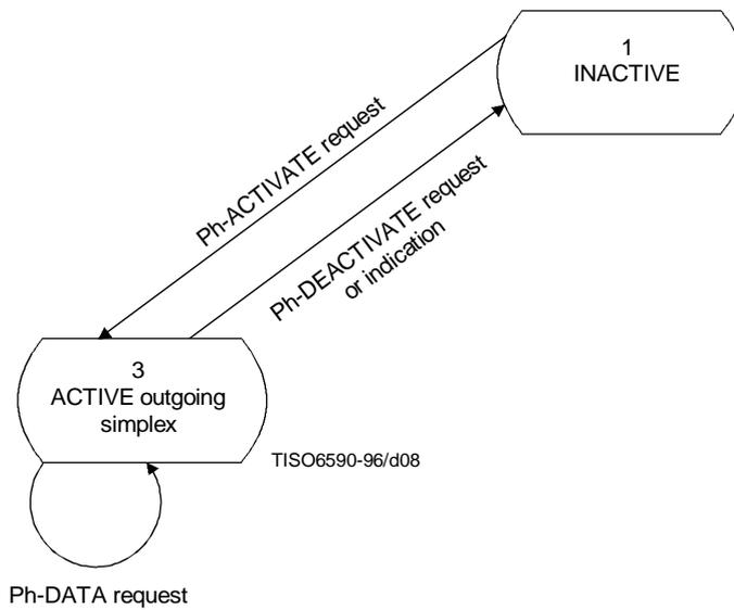
Figure 7 – State transition diagram for simplex mode, outgoing
