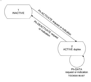
Figure 6 – State transition diagram for duplex mode with Activation/Deactivation
