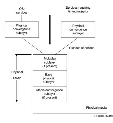
Figure A.1 – Structure of the Physical Layer
