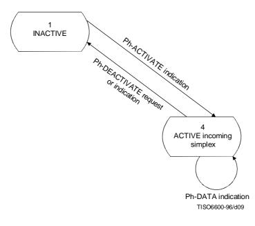
Figure 8 – State transition diagram for simplex mode, incoming
