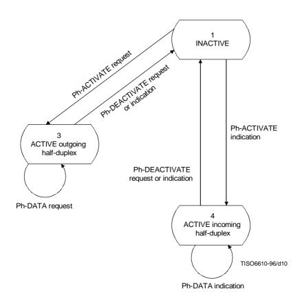
Figure 9 – State transition diagram for half-duplex mode
