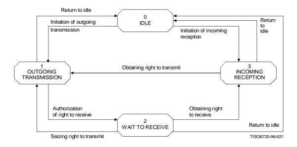
Figure B.2 – State diagram for HDM
