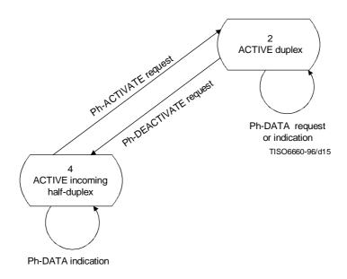
Figure 14 - State transition diagram for half-duplex/duplex mode shift
