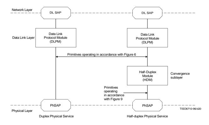
Figure B.1 – Structure of the data link layer
