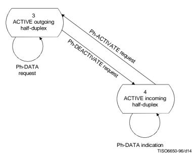
Figure 13 – State transition diagram for half-duplex mode without inactive state
