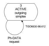
Figure 11 – State transition diagram for simplex mode, outgoing, data transfer phase only
