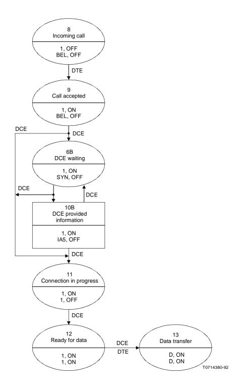
$FIGURE\ A-6/X.21$  Call control phase for called DTE with simple sub-addressing for the Circuit-switched service
