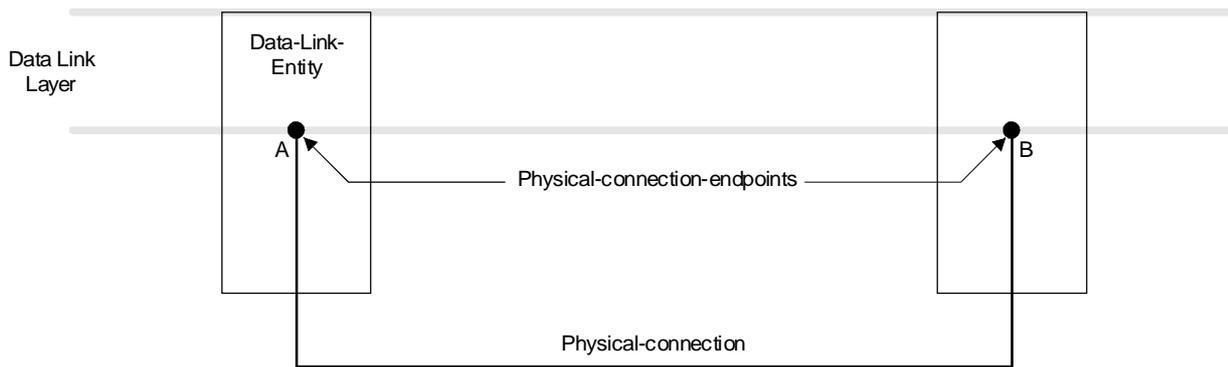
a) Example of a two endpoint physical connection
