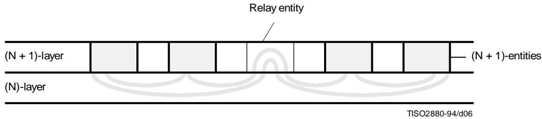
**Figure 6 – Communication through a relay**
