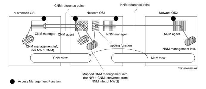
Figure 4/X.170 – Functional architecture of NNM
