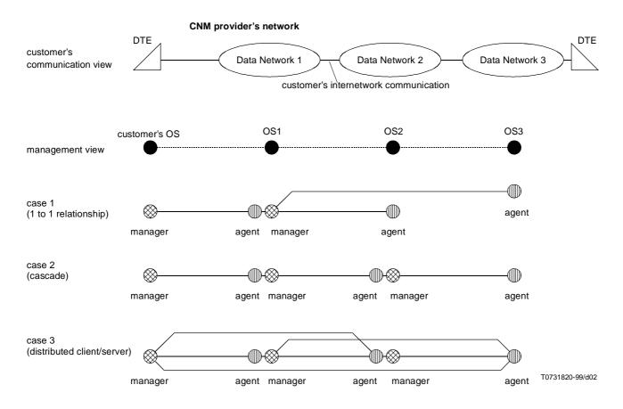
Figure 2/X.170 – Modelling for the case involving multiple networks
