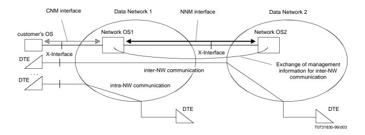
Figure 3/X.170 – Physical architecture of NNM
