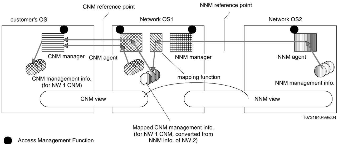
**Figure 4/X.170 – Functional architecture of NNM**
