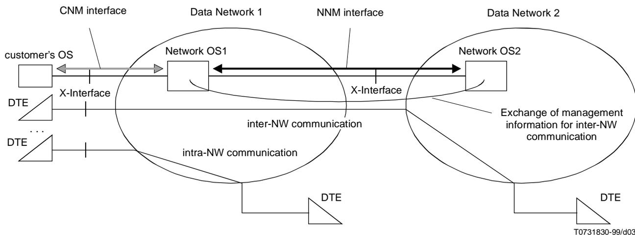
**Figure 3/X.170 – Physical architecture of NNM**
