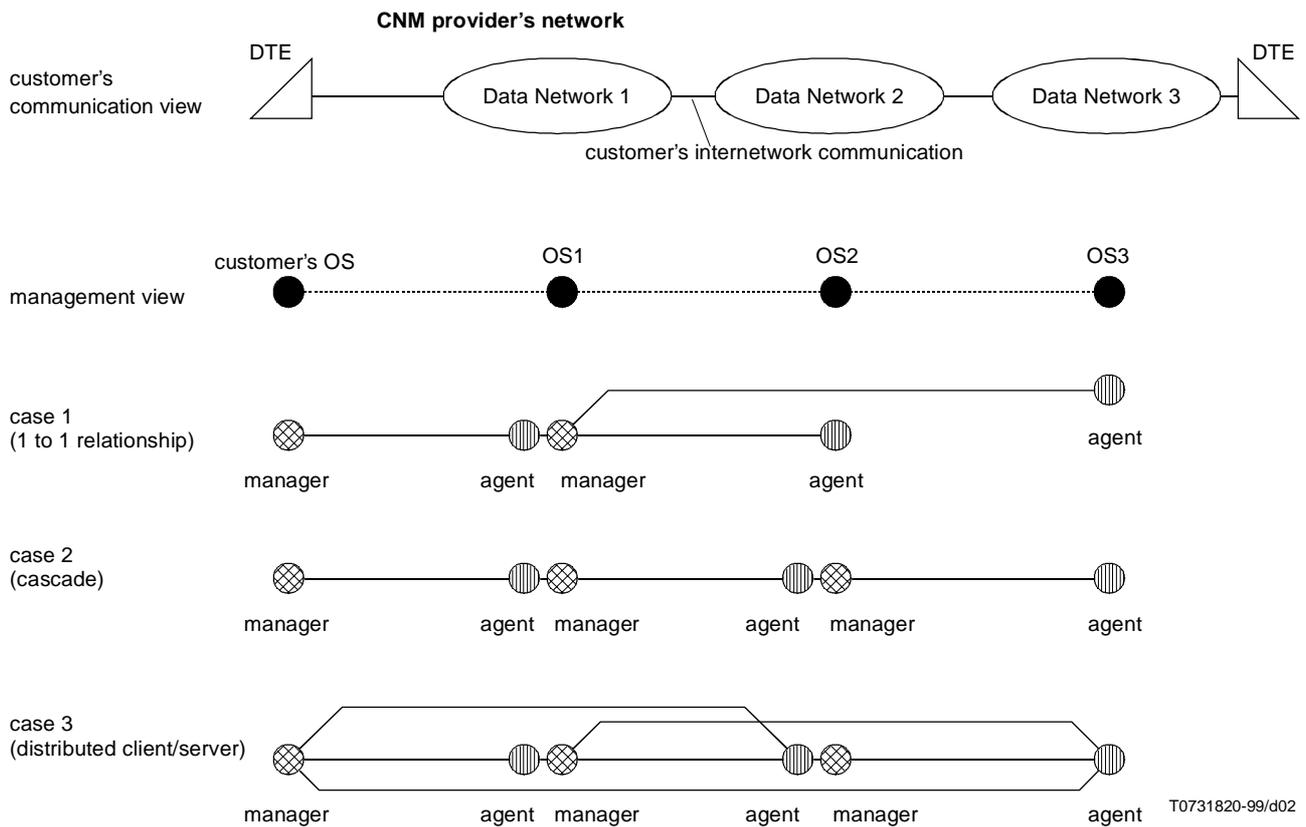
**Figure 2/X.170 – Modelling for the case involving multiple networks**
