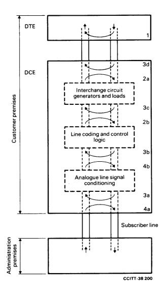
Note – The back-to-back loopbacks (e.g. 3d/2a. 3c/2b. 3b/4b and 3a/4a) that are provided should be configured in such a manner that there is no active equipment between the loopbacks. For example: an Administration may operate the back-to-back loopbacks simultaneously in the same relay or switch.
