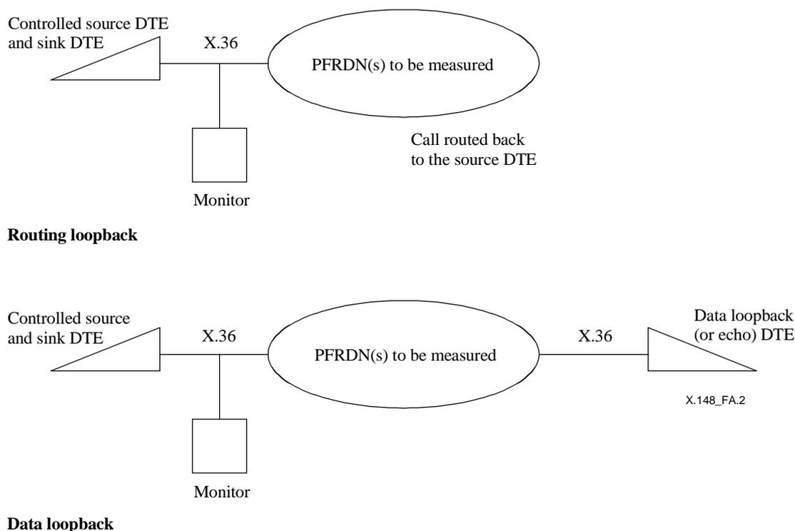
**Figure A.2/X.148 – Loopback architectures**
