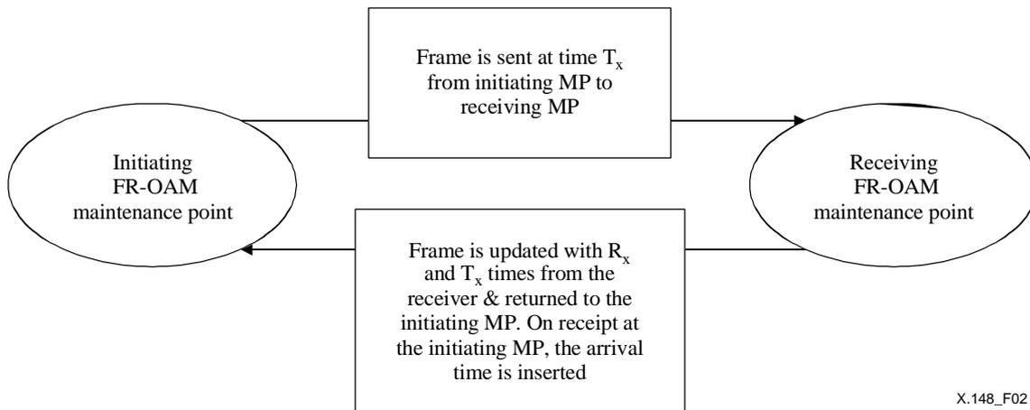
Figure 2/X.148 – Measurement of RTD using OAM frames
