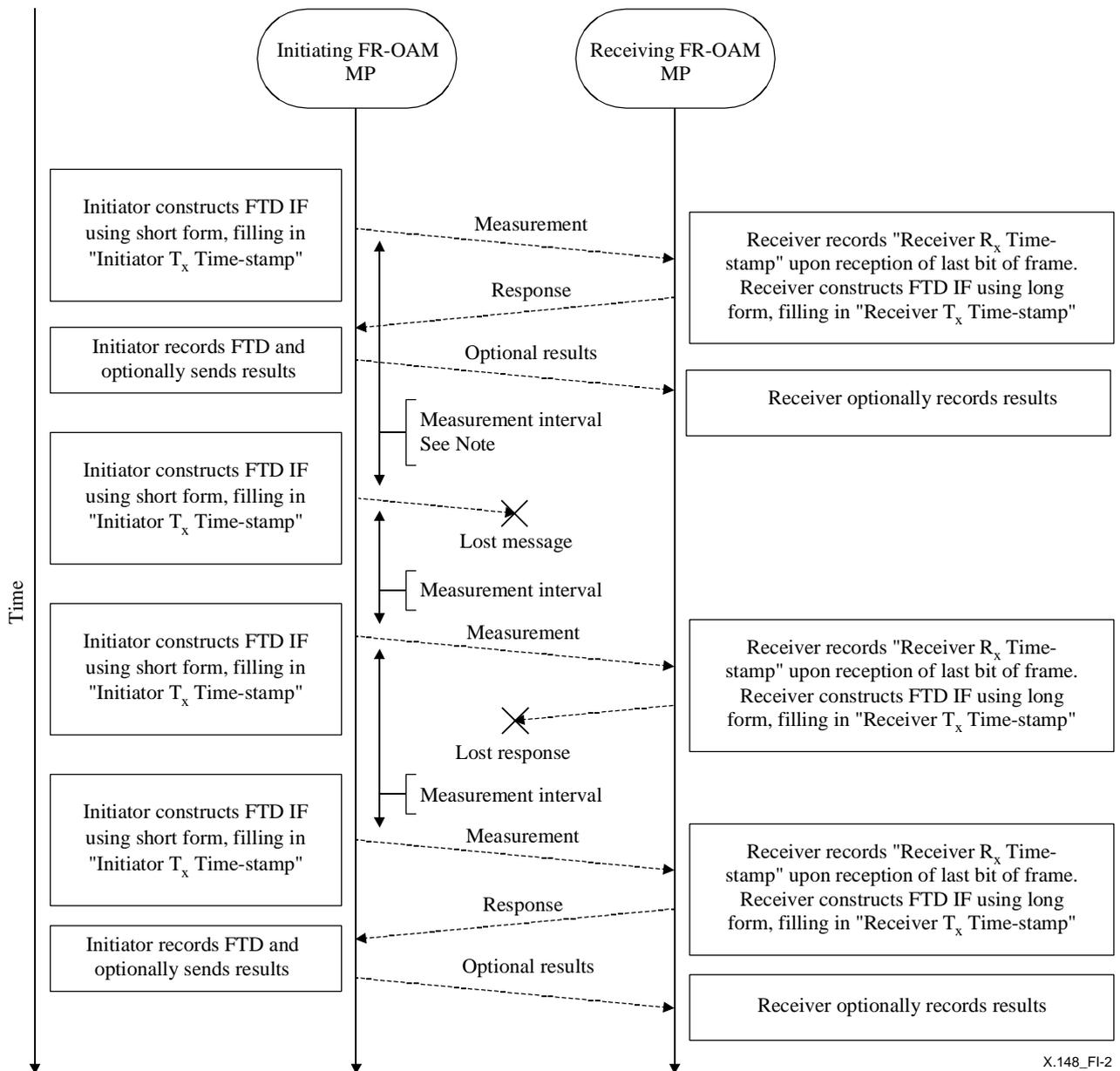
**Figure I.2/X.148 – OAM message flows for frame transfer delay measurement**
