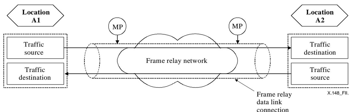
**Figure II.1/X.148 – Measurement of end-to-end data delivery ratio**
