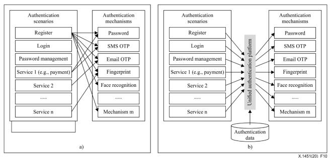
Figure 10 – Authentication scenarios and mechanisms
