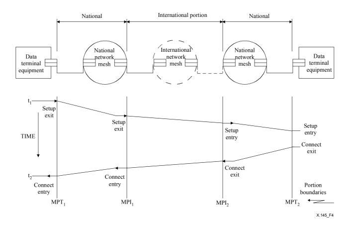
Figure 4/X.145 – Connection set-up delay at the MPT<sub>1</sub> boundary
