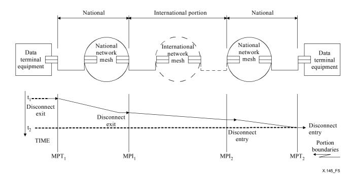
Figure 5/X.145 – End-to-end disconnect delay
