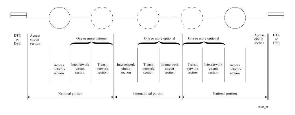
Figure 2/X.145 – Portions of an international virtual connection
