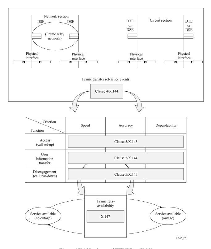
Figure 1/X.145 – Scope of ITU-T Rec. X.145
