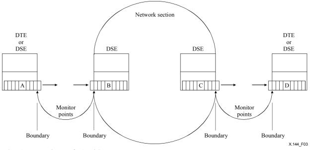
NOTE 1 – Frame exit events for A and C. NOTE 2 – Frame entry events for B and D.
