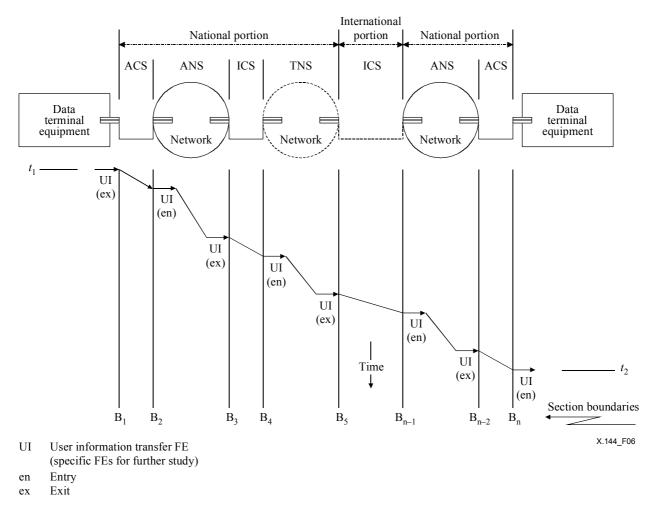
NOTE –  $(t_1 - t_2)$  may be observed on the calling side and called side of any virtual connection portion.
