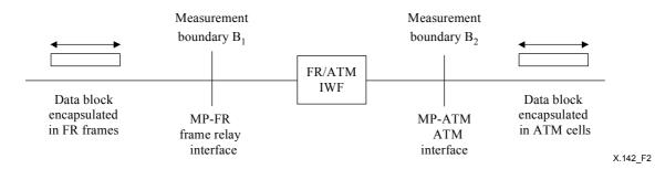
Figure 1/X.142 – Frame relay/ATM service interworking
