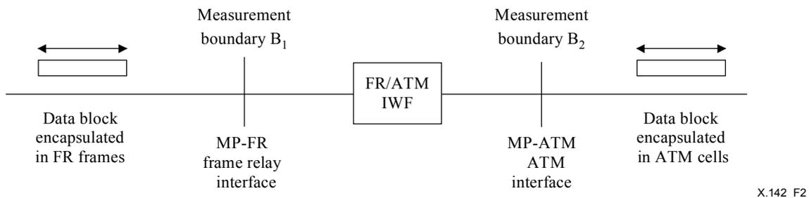
**Figure 2/X.142 – General location of measurement points**
