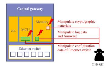
**Figure 5** – **Threats to integrity of data units under communication**
