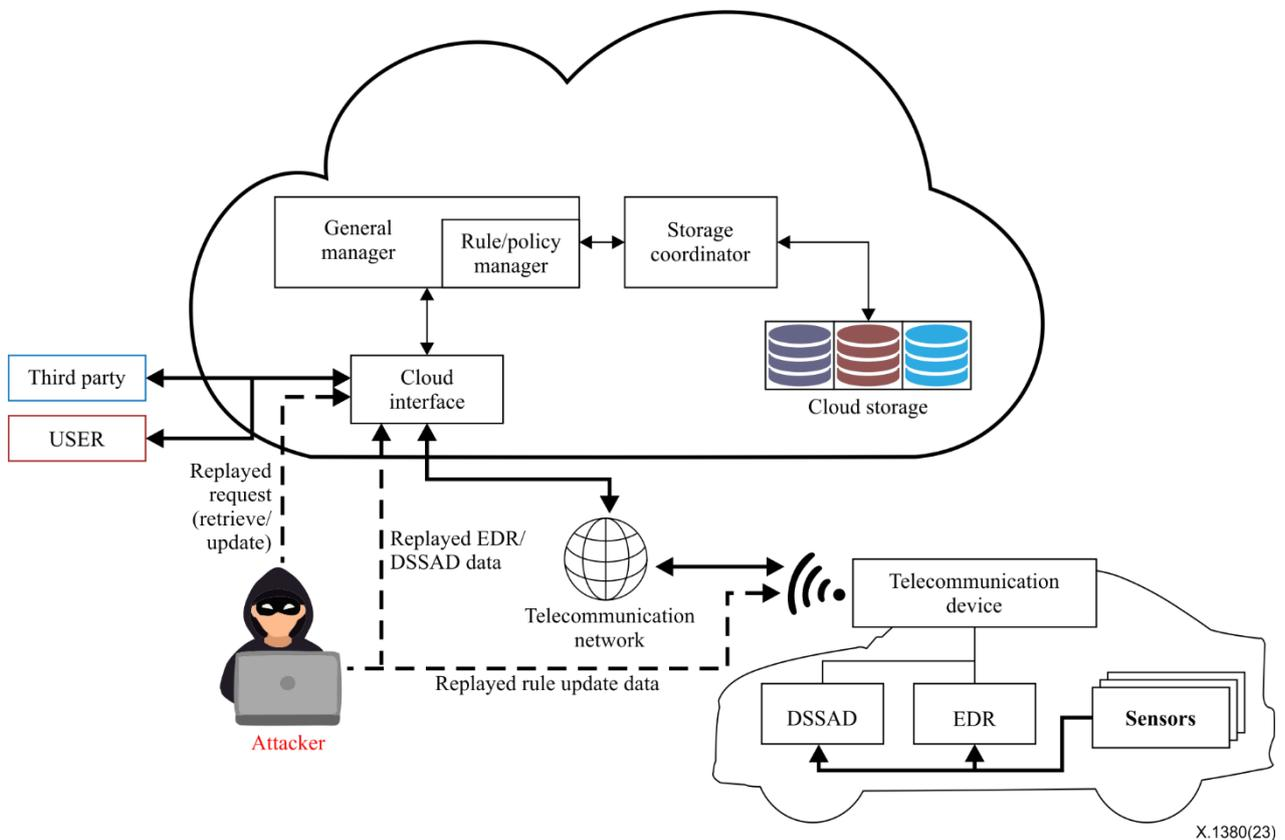
**Figure 13 – Replay attack on cloud-based data recorder systems**
