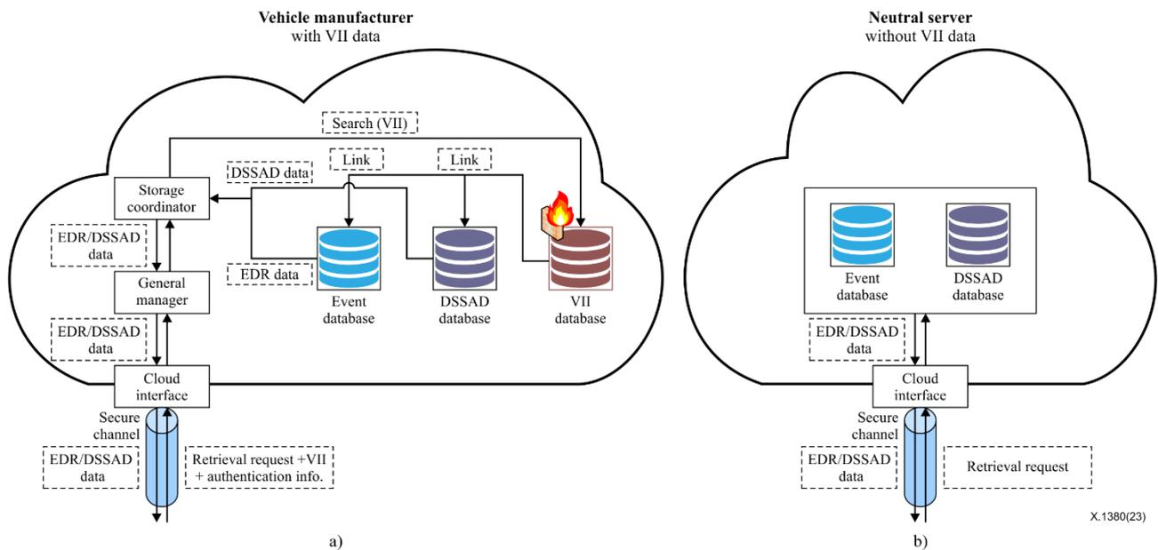
**Figure 17 – Retrieving procedure of storage separation**
