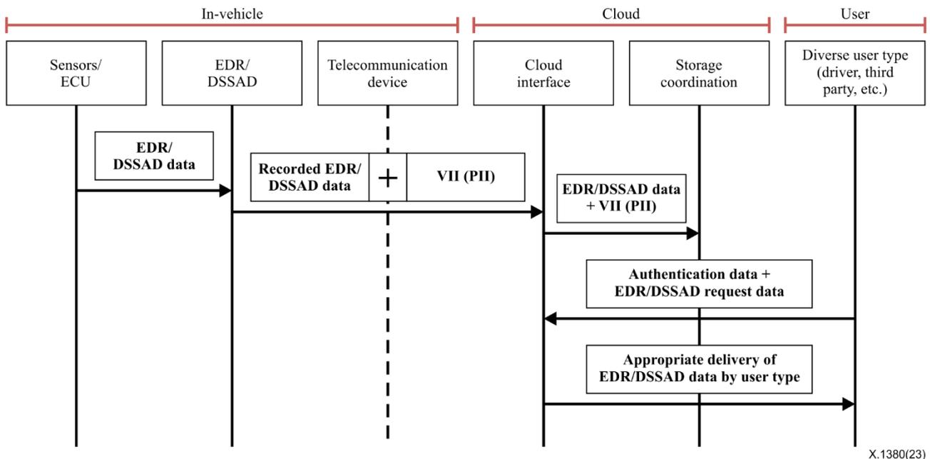
**Figure 8 – The data flow of the cloud-based EDR/DSSAD**
