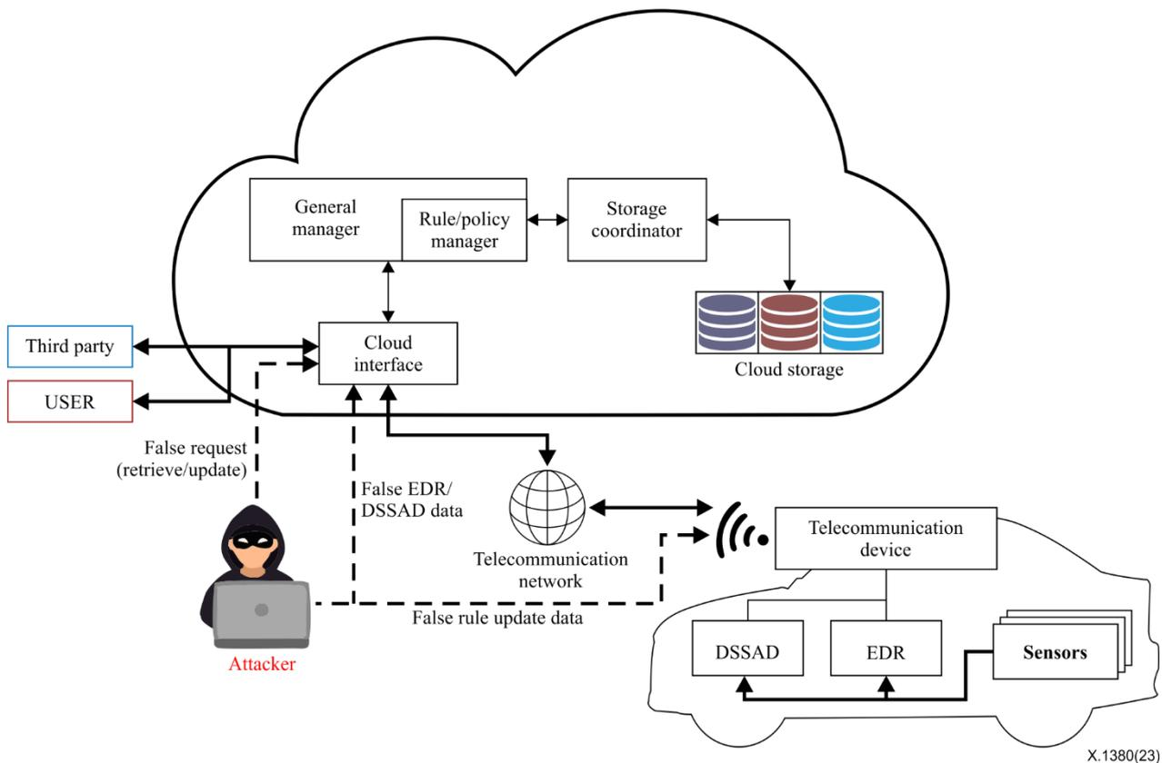
**Figure 12 – Impersonation attack on cloud-based data recorder systems**
