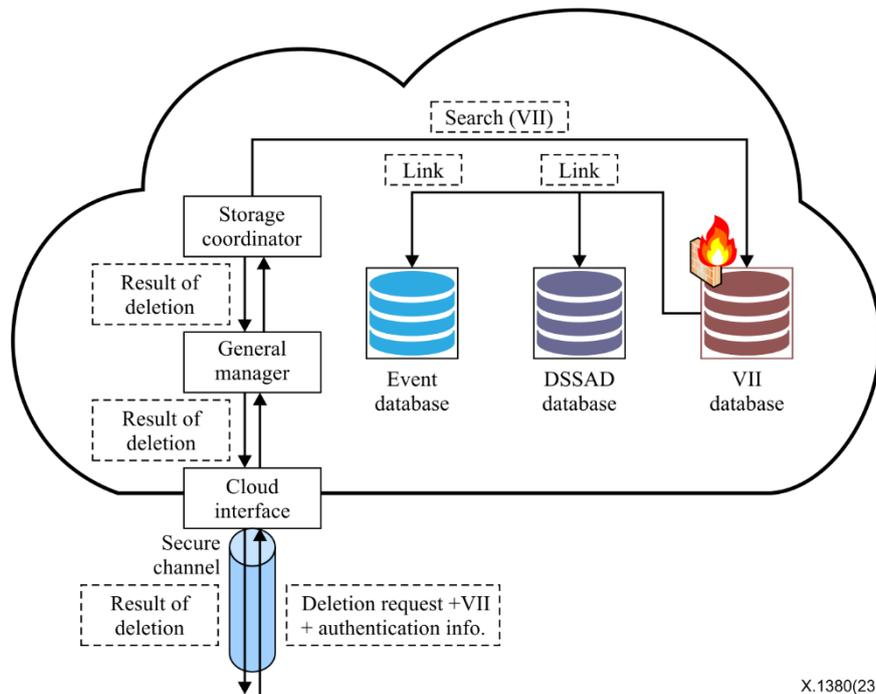
**Figure 18 – Deletion procedure of storage separation**
