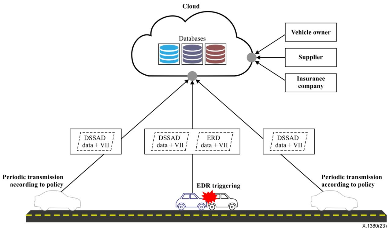
**Figure 20 – The flow of EDR/DSSAD data**
