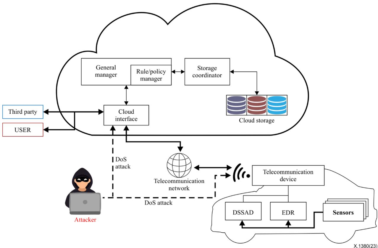
Figure 14 – DoS attack on cloud-based data recorder systems
