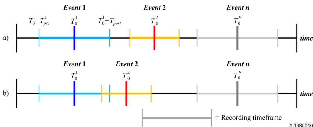
**Figure 4 – Recording timeframe of EDR: (a) non-overlapped events (b) overlapped events**
