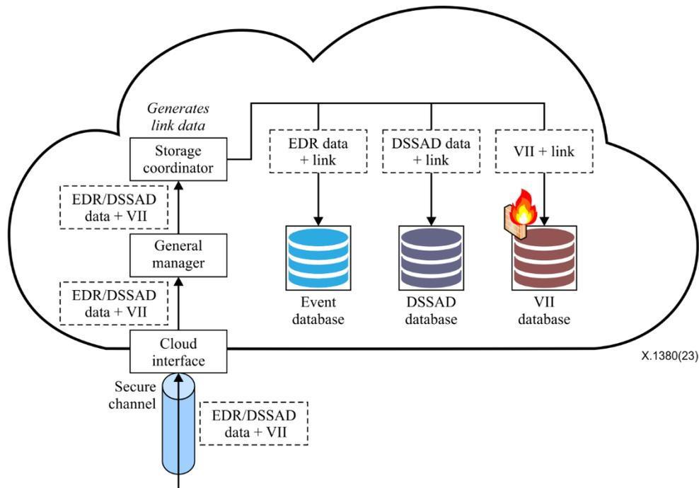
**Figure 16 – Storing procedure of storage separation**
