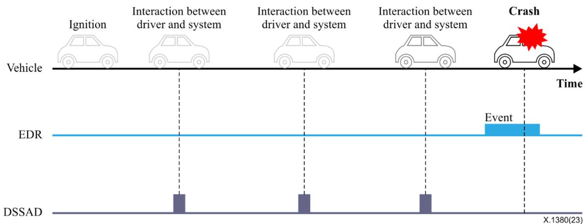
Figure 6 – Data recording time of EDR and DSSAD
