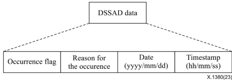
**Figure 7 – The data format of DSSAD**
