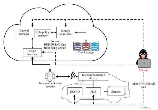
Figure 11 – Manipulate the control flow on cloud-based data recorder systems
