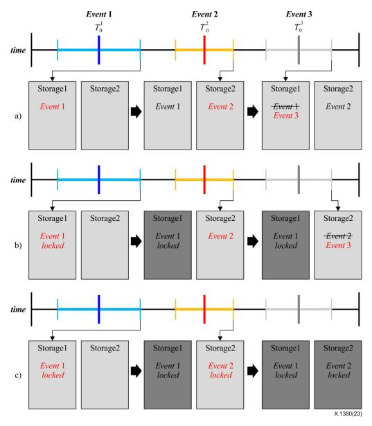
Figure 5 – Example of EDR recording with two storages: (a) without data lock, (b) with data lock condition only for Event 1, (c) with data lock condition both for Event 1 and Event 2
