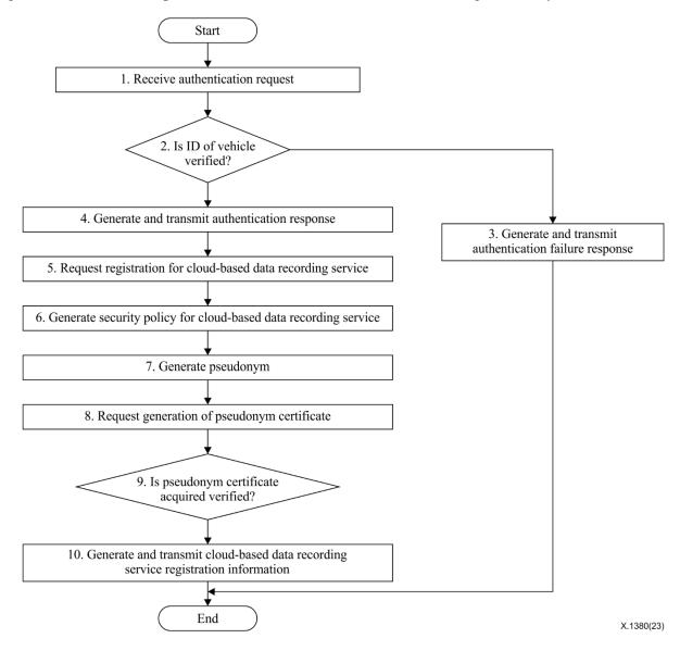
Figure 19 – Cloud-based data recording service registration
