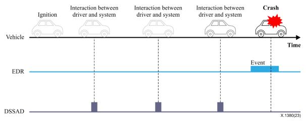
Figure 6 – Data recording time of EDR and DSSAD
