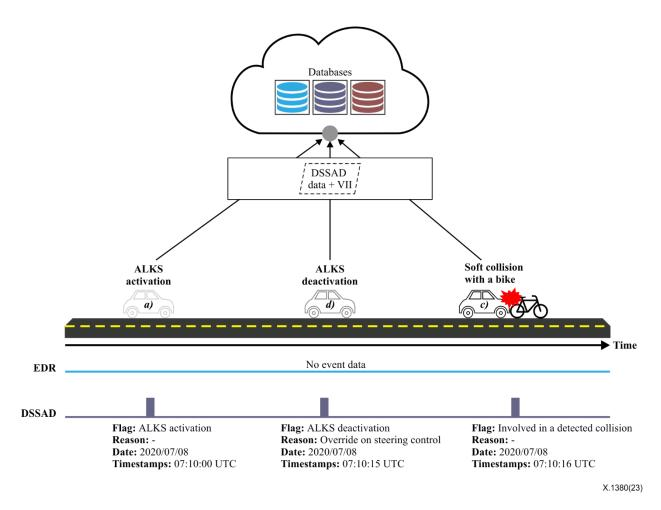
Figure 22 – A crash between a vehicle and bike
