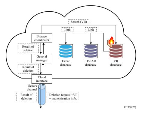
**Figure 18 – Deletion procedure of storage separation**
