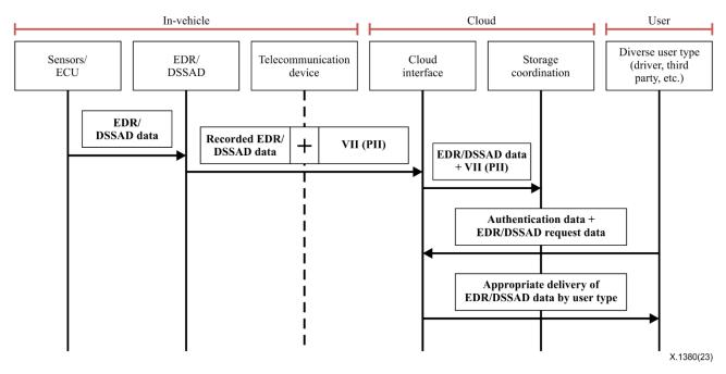
Figure 8 – The data flow of the cloud-based EDR/DSSAD
