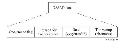
Figure 7 – The data format of DSSAD
