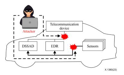
Figure 10 – Wiretapping on cloud-based data recorder systems
