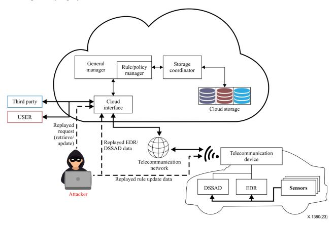
Figure 13 – Replay attack on cloud-based data recorder systems
