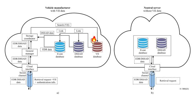
**Figure 17 – Retrieving procedure of storage separation**
