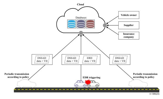
Figure 20 – The flow of EDR/DSSAD data
