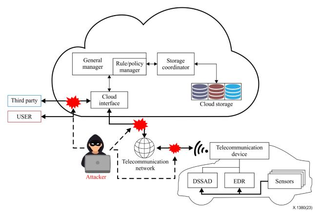
Figure 9 – Eavesdropping on cloud-based data recorder systems
