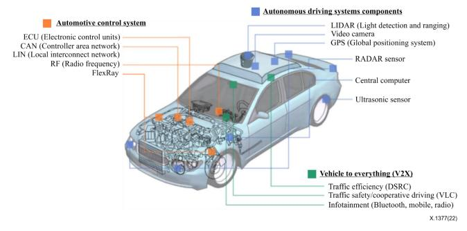
Figure 1 – Overall attack surface for connected vehicles
