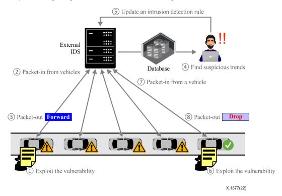
Figure I.5 – Procedure for incident response for connected vehicles
