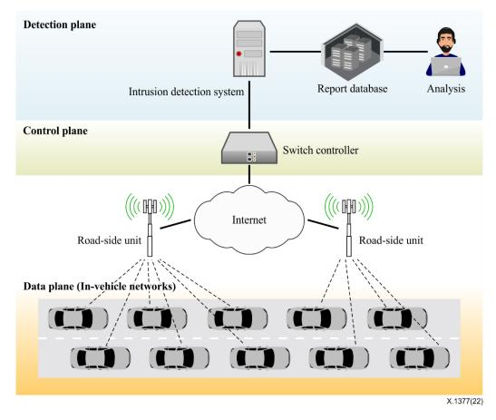
Figure 2 – Intrusion prevention system for connected vehicles
