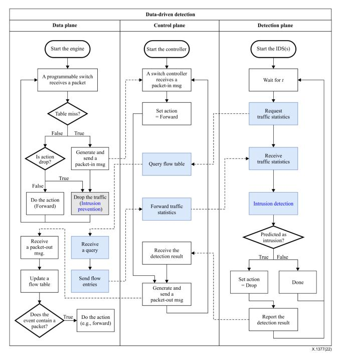
Figure 8 – Data-driven detection method
