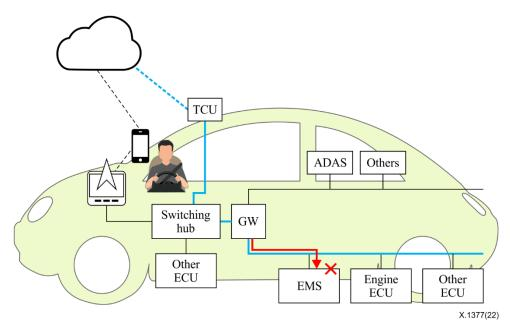
Figure I.3 – Procedure when an engine management system is compromised
