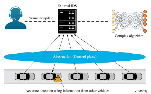
Figure 4 – External intrusion detection system and its characteristics
