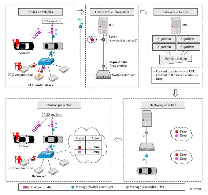
**Figure 6 – Illustration of the intrusion prevention procedure**
