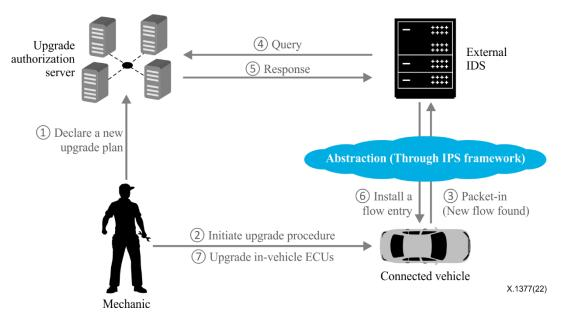
Figure I.4 – Procedure for in-vehicle electronic control unit firmware upgrade
