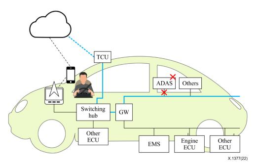
Figure I.2 – Procedure when an advanced driver assistance system unit is compromised
