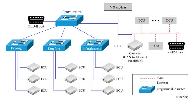
Figure 3 – Configuration of an in-vehicle network and programmable switches
