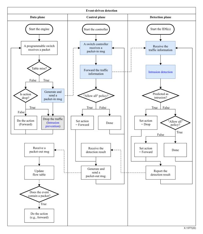
Figure 7 – Event-driven detection method
