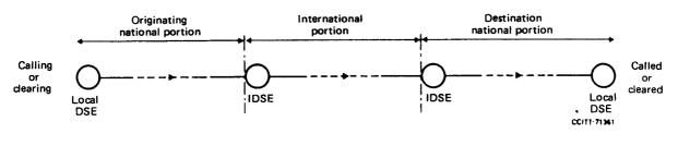
Note 1 – A DSE may also function as an IDSE. Note 2 – Arrows indicate direction of call set-up or clear-down.
