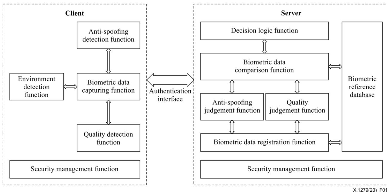
**Figure 1 – Architectural diagram of enhanced authentication using telebiometrics with ASD mechanisms**
