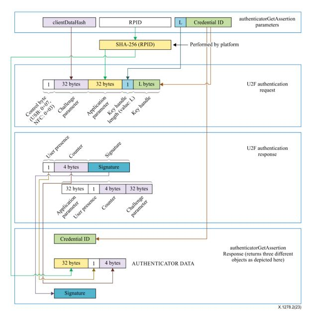
Figure 4 – Mapping: WebAuthn authenticatorGetAssertion to and from CTAP1/U2F authentication messages
