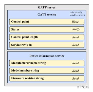
Figure 5 – Mandatory GATT services and characteristics that MUST be offered by an authenticator
