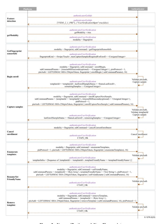
Figure 2 – User verification modality – Fingerprint
