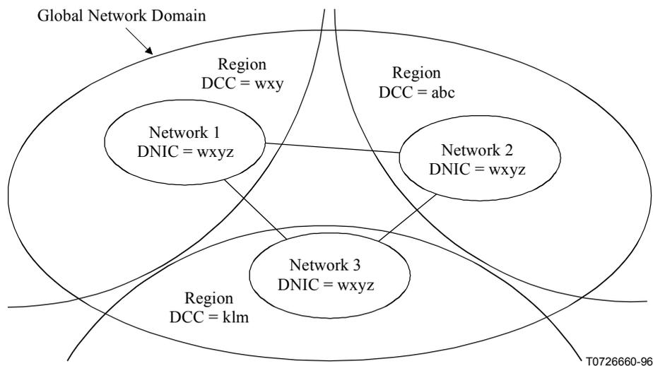
**Figure H.2/X.121 – Global network composed of subnetworks identified by a common DNIC allocated to the parent network**
