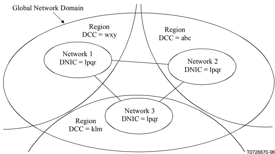
**Figure H.3/X.121 – Global network composed of subnetwork identified by a common DNIC = 1pqr allocated from the global series**
