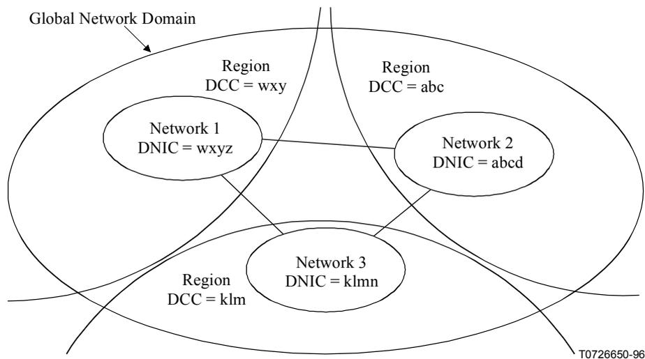
**Figure H.1/X.121 – Global network composed of subnetworks identified by a DNIC appropriate to the region in which the subnetwork operates**
