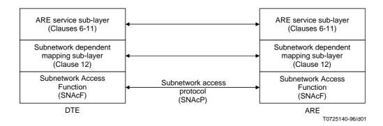
FIGURE 1/X.116 Subdivision of network layer into sub-layers
