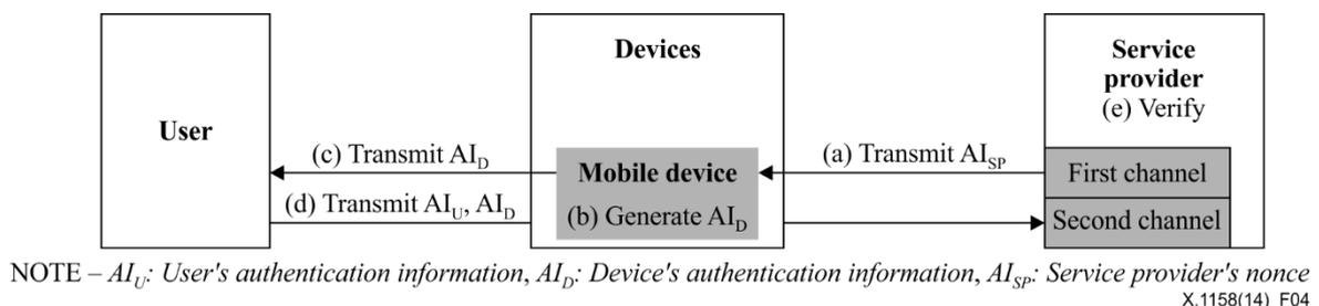
**Figure 4 – Bidirectional multiple channels model**
