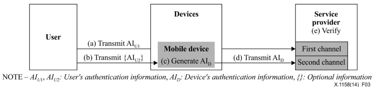
**Figure 3 – One-directional multiple channels model**
