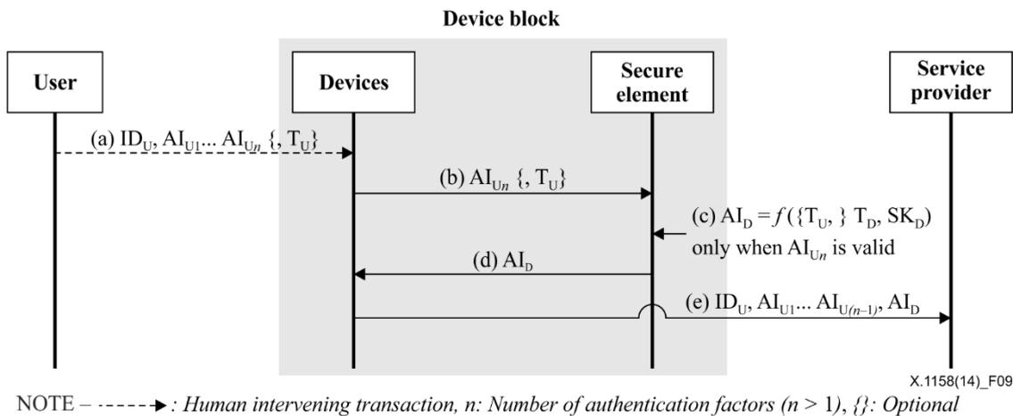
**Figure 9 – Protocol for the mobile device with secure elements model**
