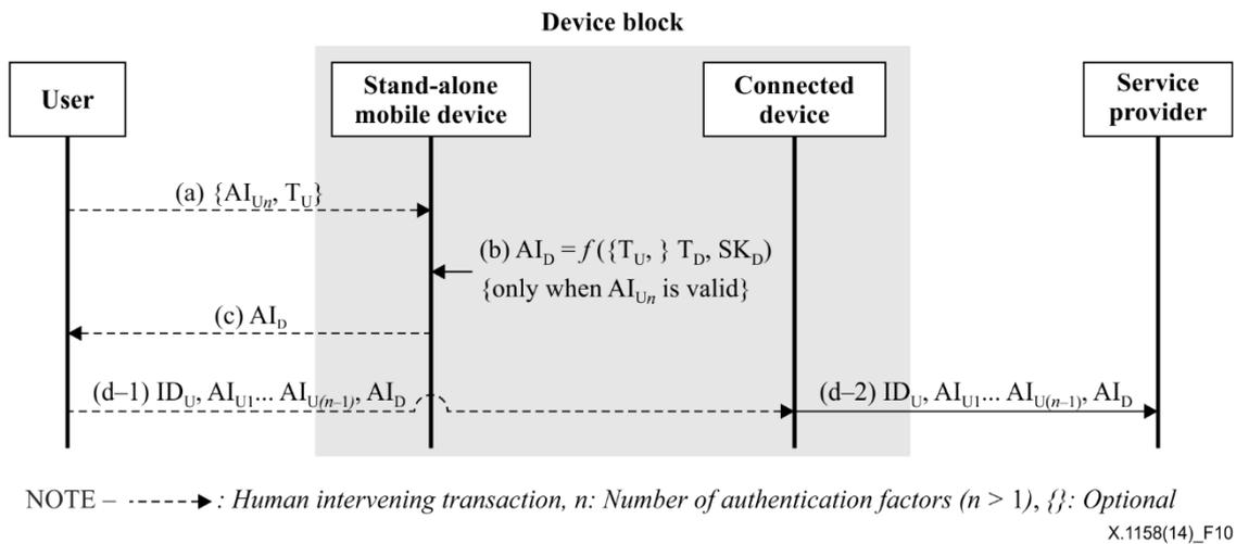
**Figure 10 – Protocol for the stand-alone mobile device model**
