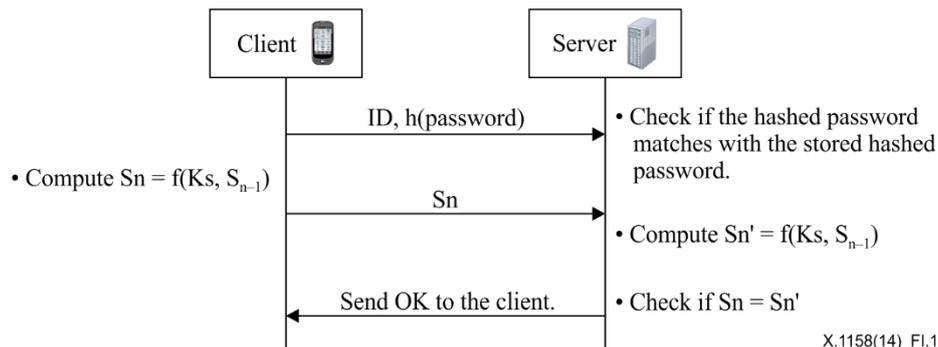
Figure I.1 – Typical two-factor authentication mechanism
