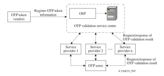
**Figure 7 – OTP management model for the centralized management framework**
