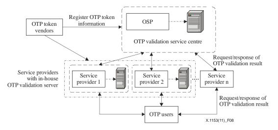
Figure 8 – OTP management model for the enhanced centralized management framework
