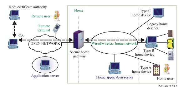
Figure 6-1 – Device authentication model for the secure home network
