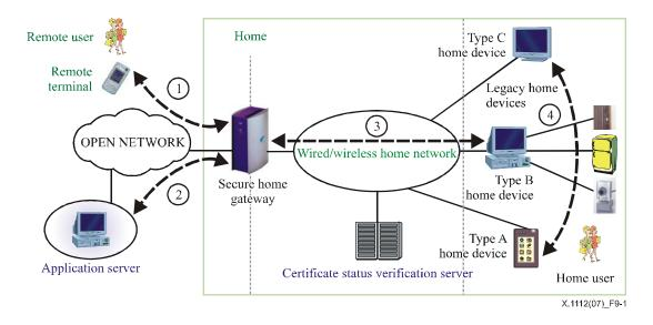
Figure 9-1 – Device authentication use case based on general home network model for security
