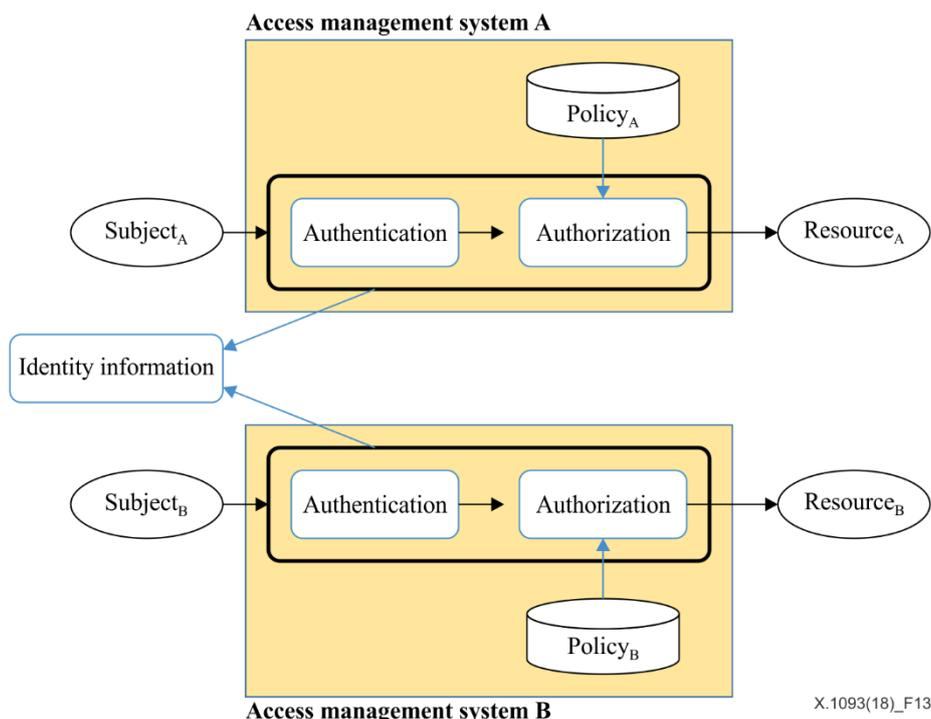
Figure 13 – Telebiometric access model with shared identity information
