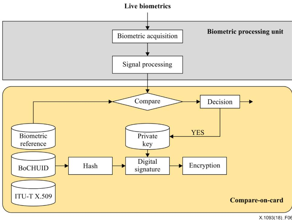
**Figure 6 – Compare-on-card with digital signature function**
