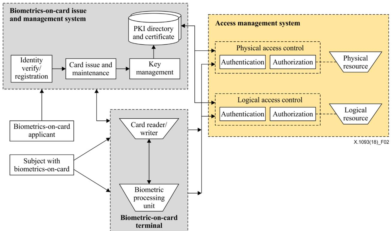
**Figure 2 – Access management with biometrics-on-card**
