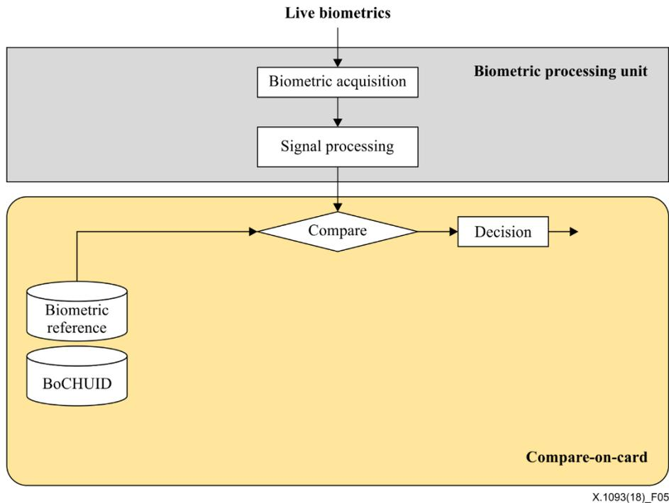
**Figure 5 – Compare-on-card without digital signature function**
