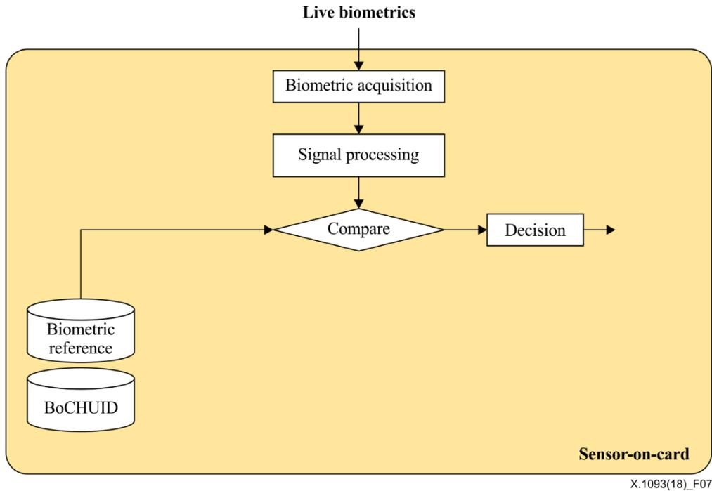
Figure 7 – Sensor-on-card without digital signature function
