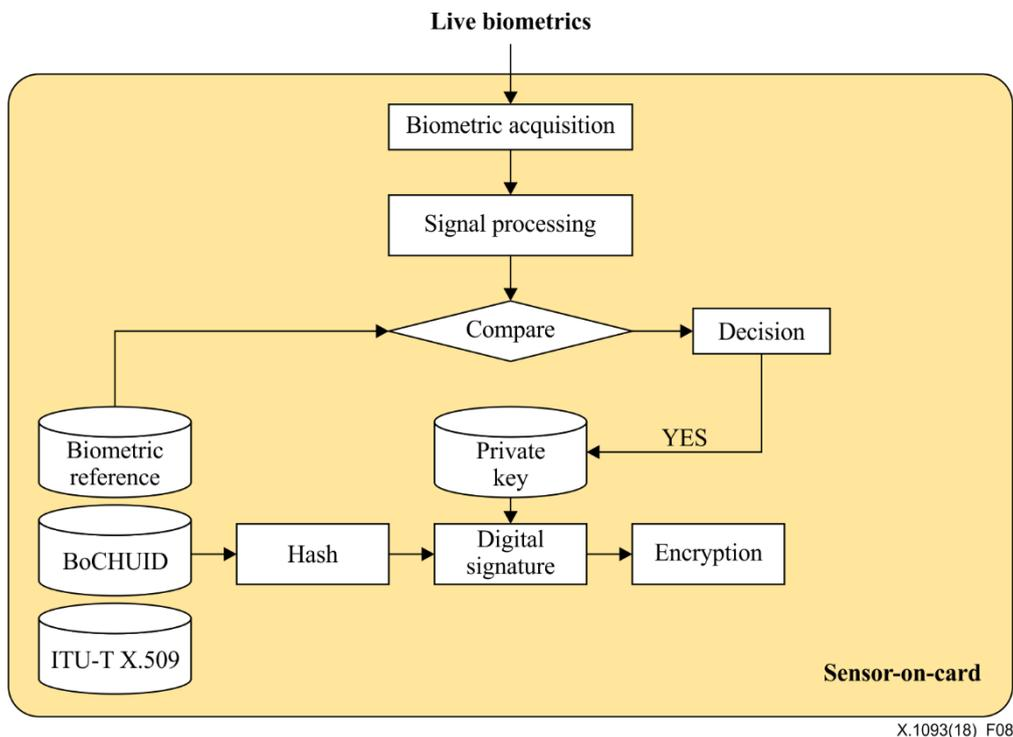
Figure 8 – Sensor-on-card with digital signature function
