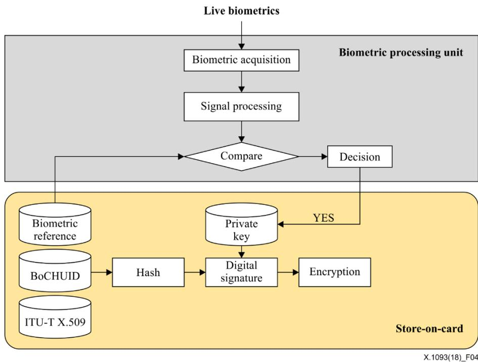
**Figure 4 – Store-on-card with digital signature function**
