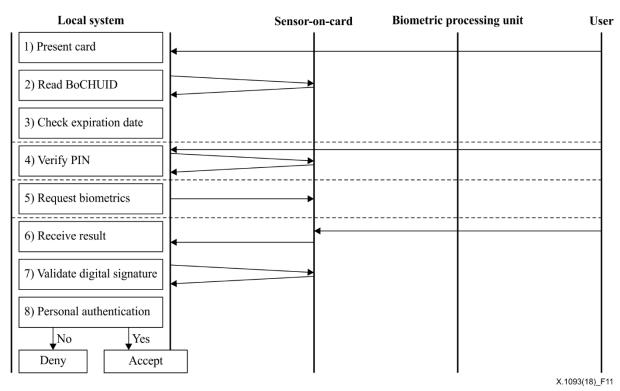
Figure 11 – Personal authentication using sensor-on-card
