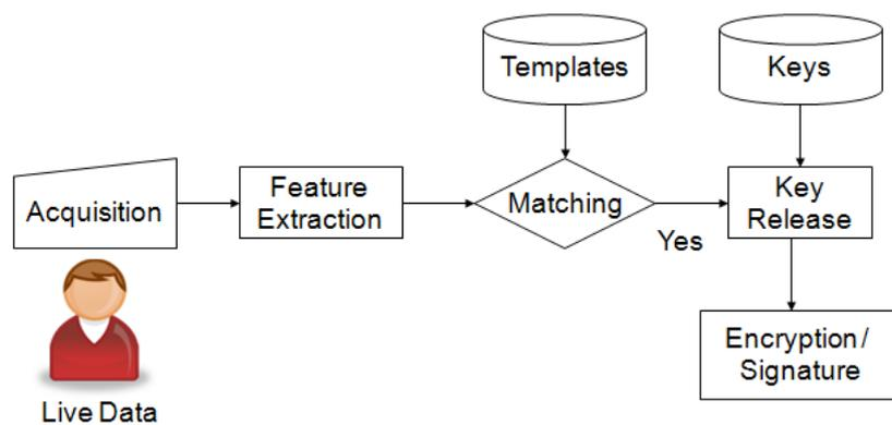
**Figure 2 – Biometric key release model**
