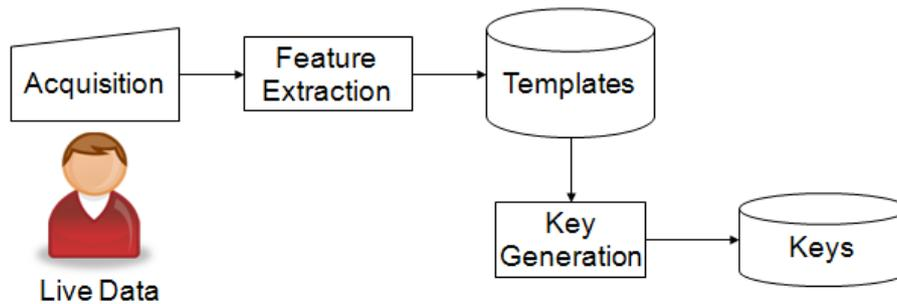
**Figure 1 – Biometric key binding/generation model**
