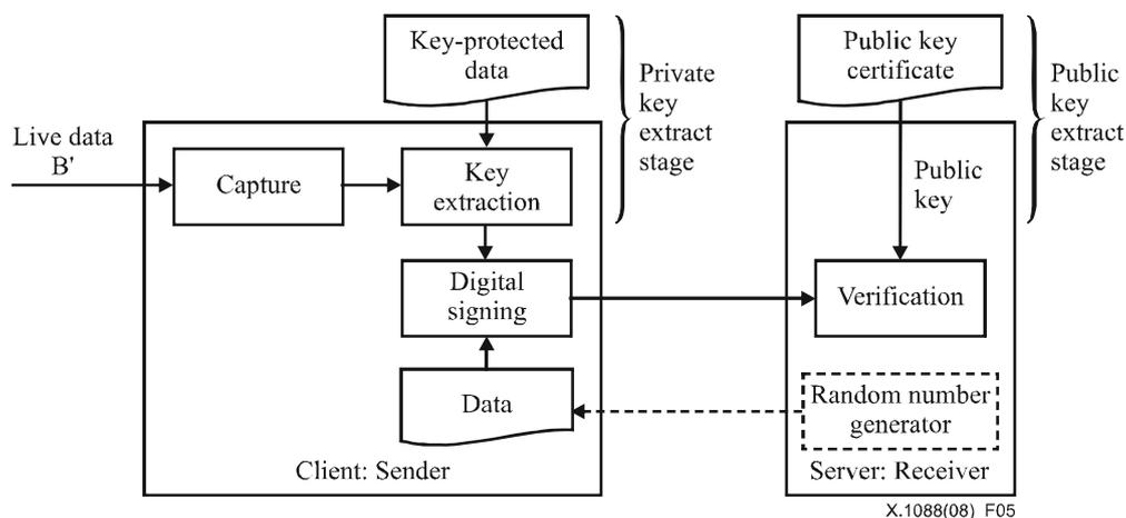
Figure 5 – Biometric digital signature framework with biometric digital key
