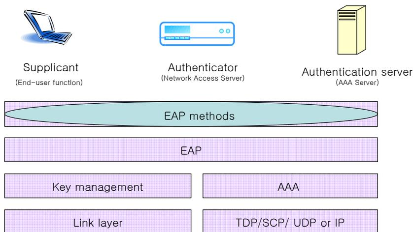
**Figure 1 – EAP-based authentication and key management framework**
