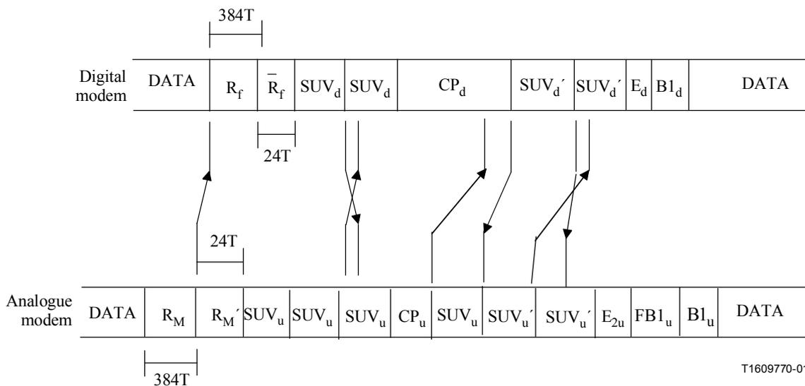
Figure 19/V.92 – Fast parameter exchange initiated by the analogue modem
