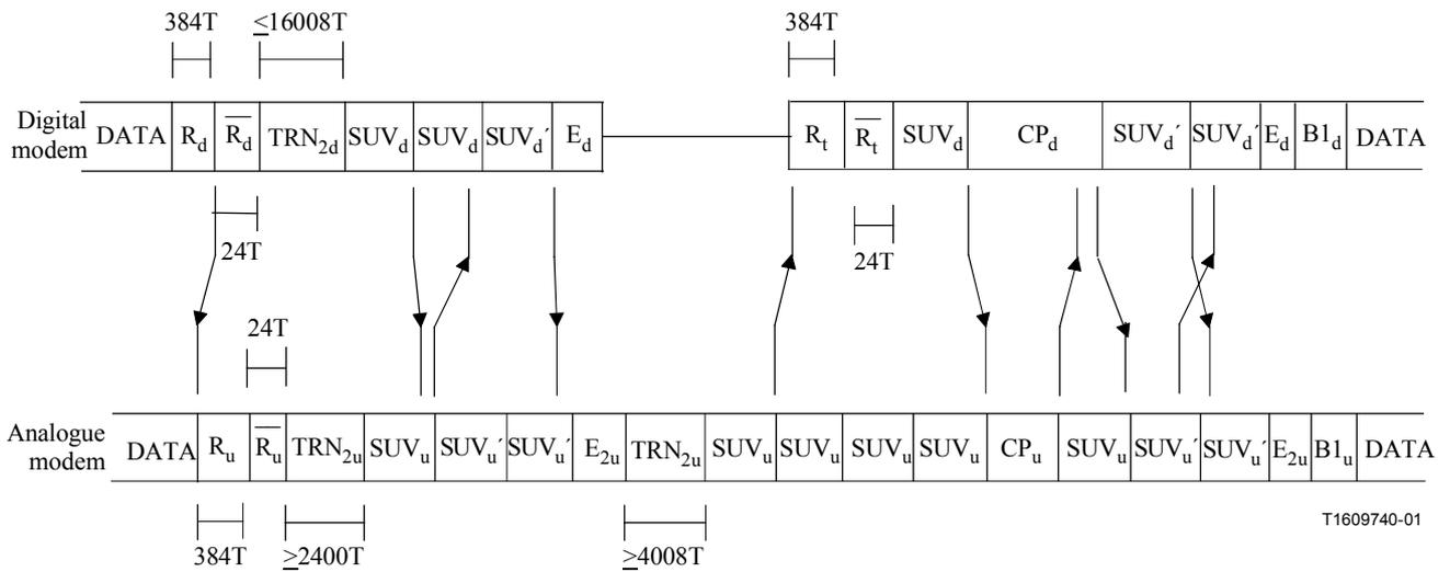
**Figure 16/V.92 – Rate renegotiation with silence requested by the digital modem and sustained for the maximum length**
