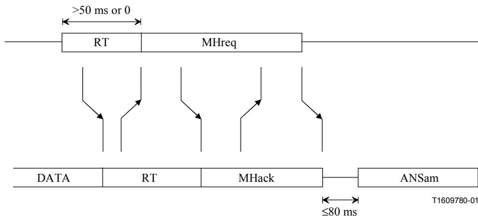
**Figure 20/V.92 – Modem-on-hold request acknowledged**
