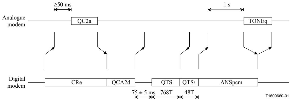
**Figure 5/V.92 – Short Phase 1 when calling modem is analogue modem and answering modem transmits CRe**
