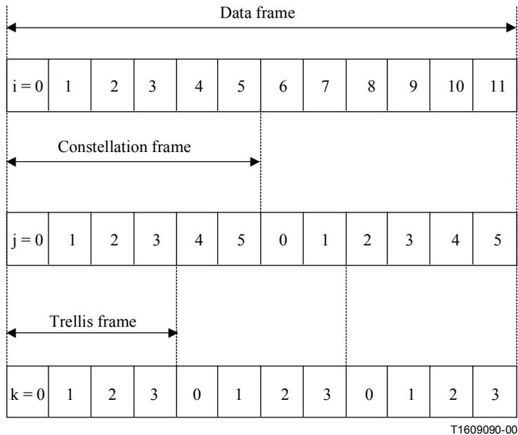
**Figure 1/V.92 – Framing structure for the analogue modem**
