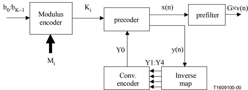
**Figure 2/V.92 – Analogue modem transmitter block diagram**
