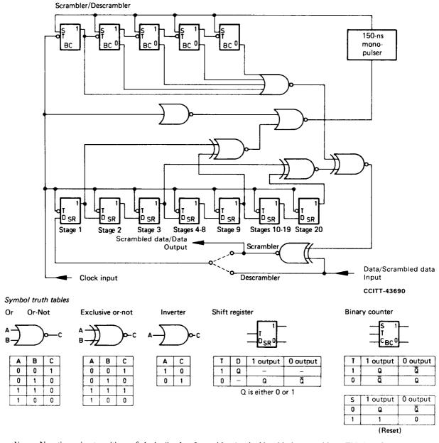
Note - Negative-going transitions of clocks (i.e. 1 to 0 transitions) coincide with data transitions. This is self-synchronizing.
